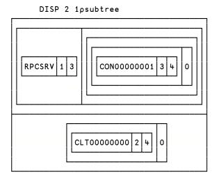
**Interpretation** There are two children of the root, named RPCSRV and CLT00000000 (this example was 'shot' while running Samples.TestRPCserver). RPCSRV is of type 1 (Server) and in state 3 (Listen). It has a child named CON00000001 which is a Connection (3) in state Connected (4). CLT00000000 is a client (2) in state Connected (4).
